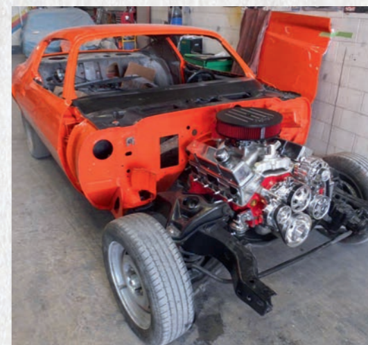
Left > Another milestone was the final fitment of the 350 to the painted body. This meant the assembly of all the front panels could be finished and the stripes could then be masked and painted.
